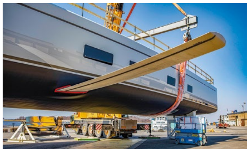
The DSS foil as it protrudes from the Baltic 142 (photo credits Eva-Stina Kjellman)
