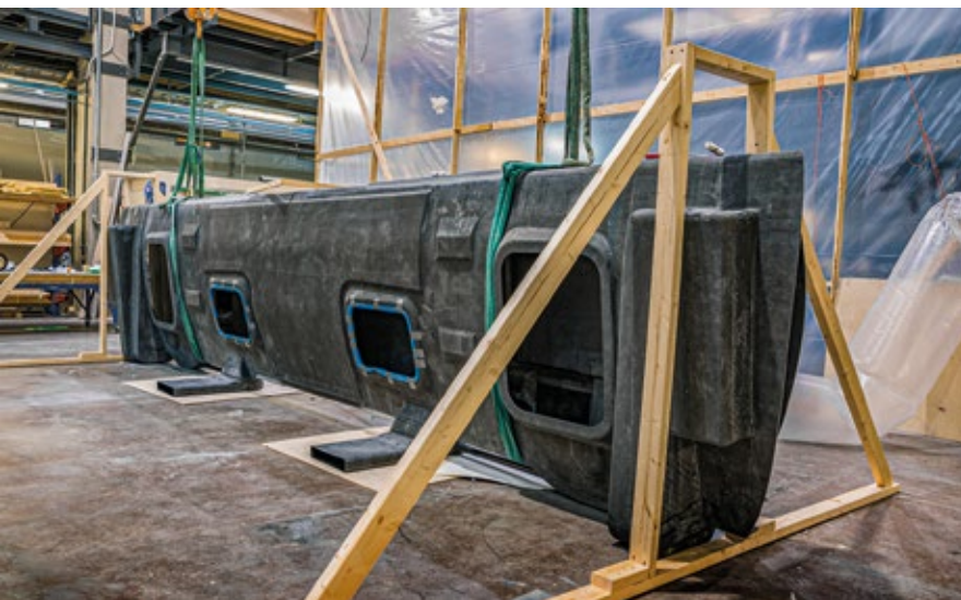
In the pictures below, Work in progress on the DSS foil container slip installed on board: notice the foil's access hatches.
